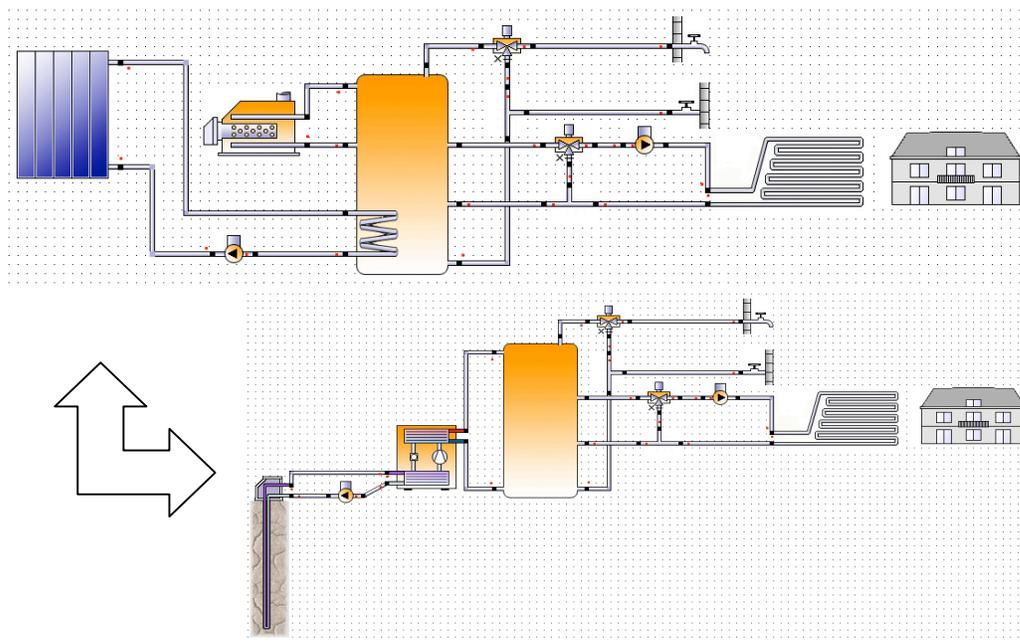
**Figure 1:** schematic comparison of a solar system and a geothermal heating system
