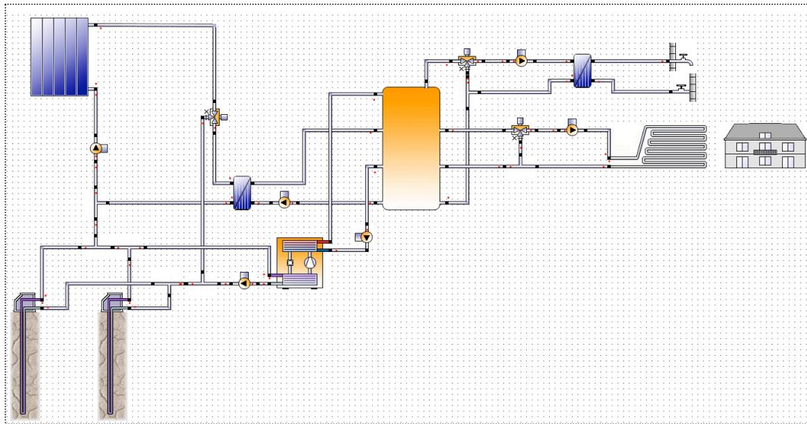
**Figure 3:** System with the capability of solar regeneration of ground-source loop fields
