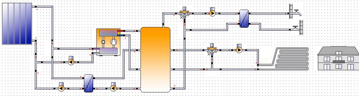
**Figure 2:** Direct connected solar thermal and heat pump system implemented in Polysun
