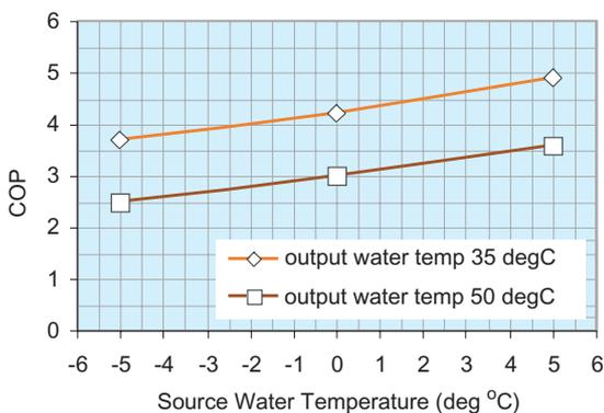
Figure 5: Coefficients of performance of typical small GSHP's
