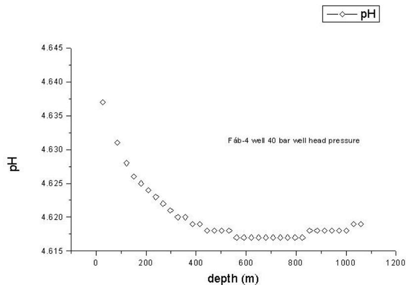
Fig. 6. The pH-depth curve in well FAB-4
