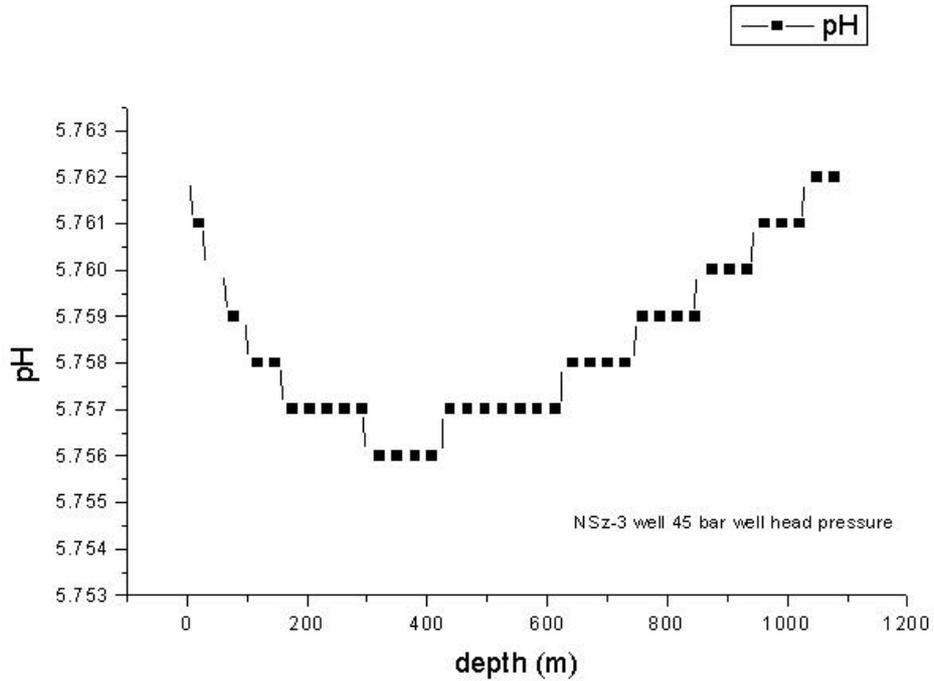
Fig.5 The pH-depth curve in well NSz-3
