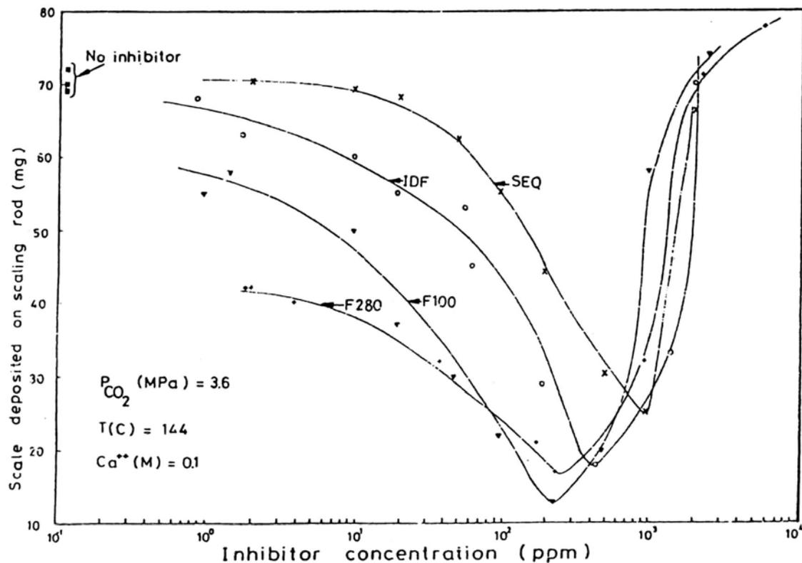
Figure 4. Scaling and inhibitor concentration
