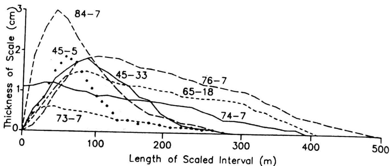
Figure 3. The normalized scale profiles in 7 US wells
