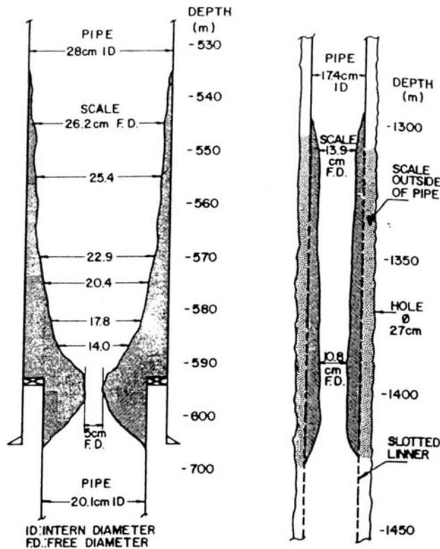
Fig.2 Typical scale profiles
