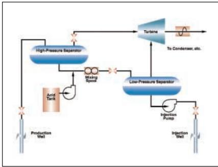
A simplified flow diagram for the pH-modification process used at some Salton Sea geothermal power plants to remove dissolved silica from the brines.
