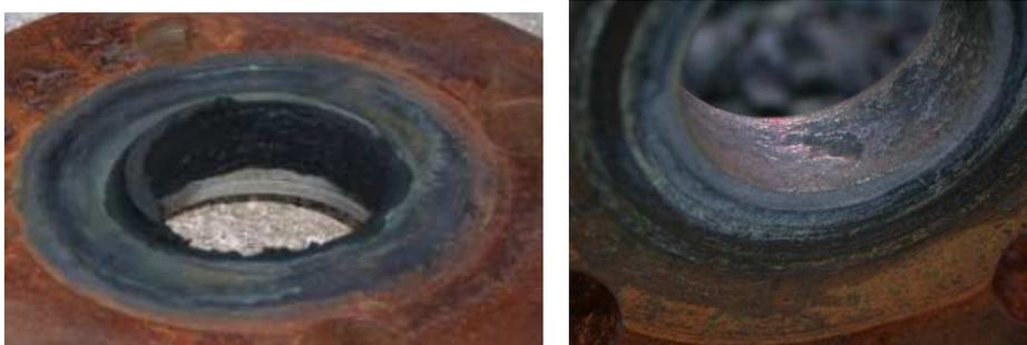
Fig. 3: corrosion morphology after 7 months exposure (left: corrosion product scale on inner surface of the electrode; right: surface after sandblasting).
